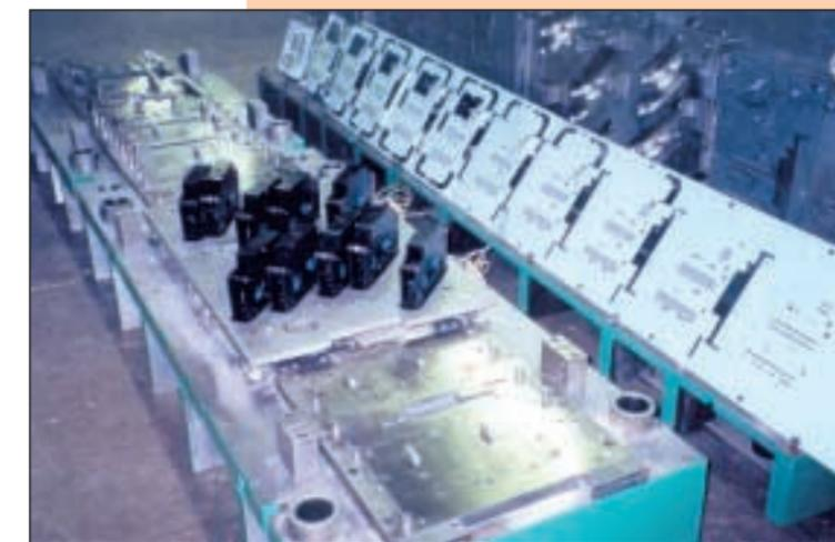
*This 10-station progressive die, with the strip showing what functions are performed at what station, incorporates tapping units, the black boxes in the center of the lower die.*
