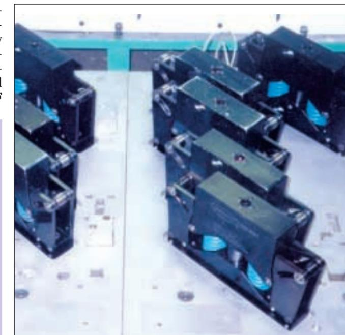
These in-die-tapping units can be removed and installed on other dies, making the technology more cost-efficient. Note the tubes in the back of the die. These supply lubrication to the tap holes during the tapping process.
